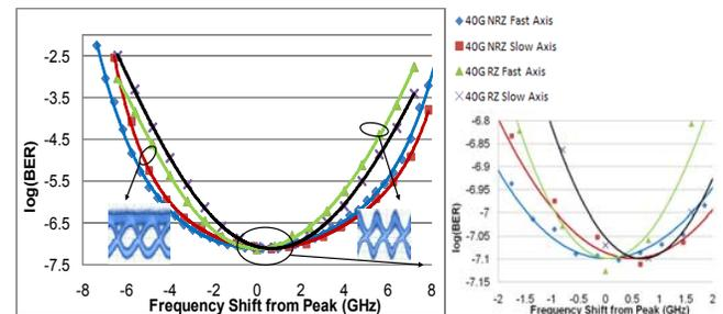
Figure 5. BER versus frequency detuning for 40G RZ and NRZ DPSK signals for the fast and slow polarization axis of a 40GHz DI.
