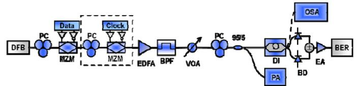
Figure 1. Schematic of the experiment setup.
