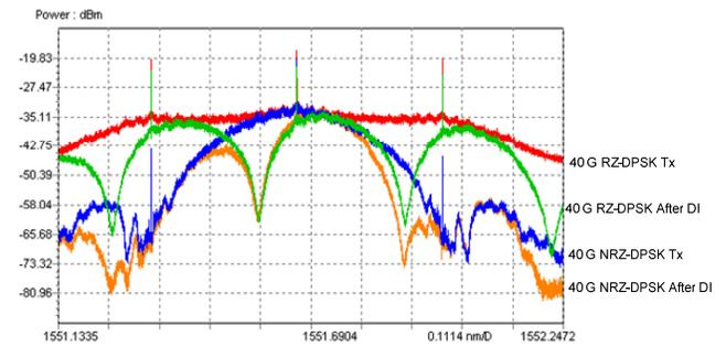
Figure 4. Comparison between 40G NRZ and RZ DPSK signals, both modulated and demodulated spectrums at a frequency offset of 11.425 GHz
