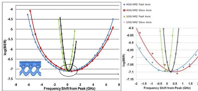
Figure 3. BER versus frequency detuning for the fast and slow polarization axis for 10 GHz and 40 GHz DI.
