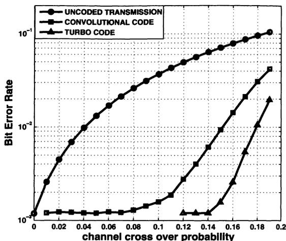
Fig. 7. Bit error rate achieved by joint decoding for (2000, 1000) turbo and convolutional codes.  $N = 4$  and  $p_s = 0.02$ .
