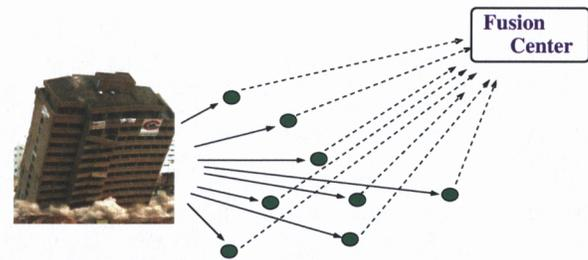
Fig. 1. A data-gathering wireless sensor network. The target data is observed by  $N$  sensors (the figure shows  $N = 8$  sensors). The sensors encode and transmit their observations to a decoder or fusion center. The decoder aims to obtain an estimate of the source.
