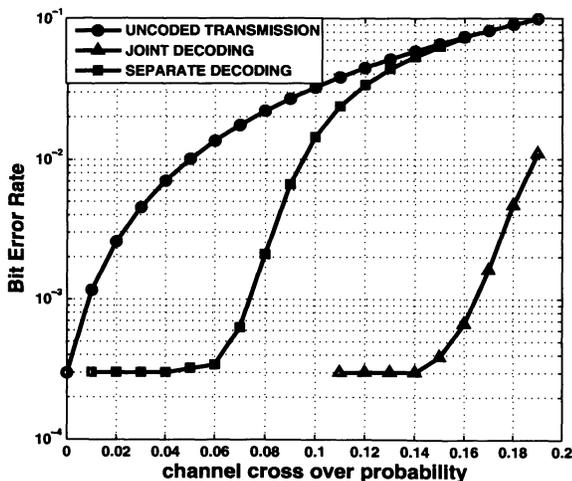
Fig. 4. Bit error rate achieved by (2000, 1000) turbo codes for  $N = 4$  sensors and  $p_s = 0.01$ .
