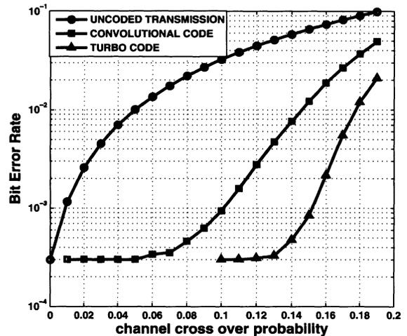
Fig. 6. Bit error rate achieved by joint decoding for (1800, 1000) turbo and convolutional codes.  $N = 4$  and  $p_s = 0.01$ .
