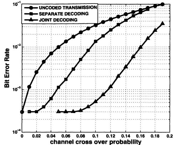
Fig. 5. Bit error rate achieved by (2000, 1000) convolutional codes for  $N = 4$  sensors and  $p_s = 0.01$ .
