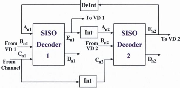
Fig. 3. Block diagram of horizontal decoder for sensor number  $n$ . VD denotes vertical decoder.
