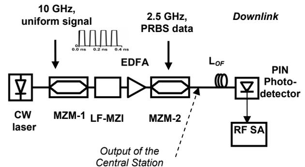
Figure 1. Schematics of the ROF link with LF-MZI.
