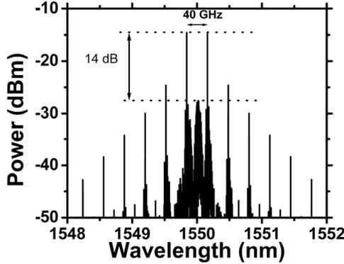
Figure 5. Optical spectrum simulated for the OCS scheme with D-LN-MZM.
