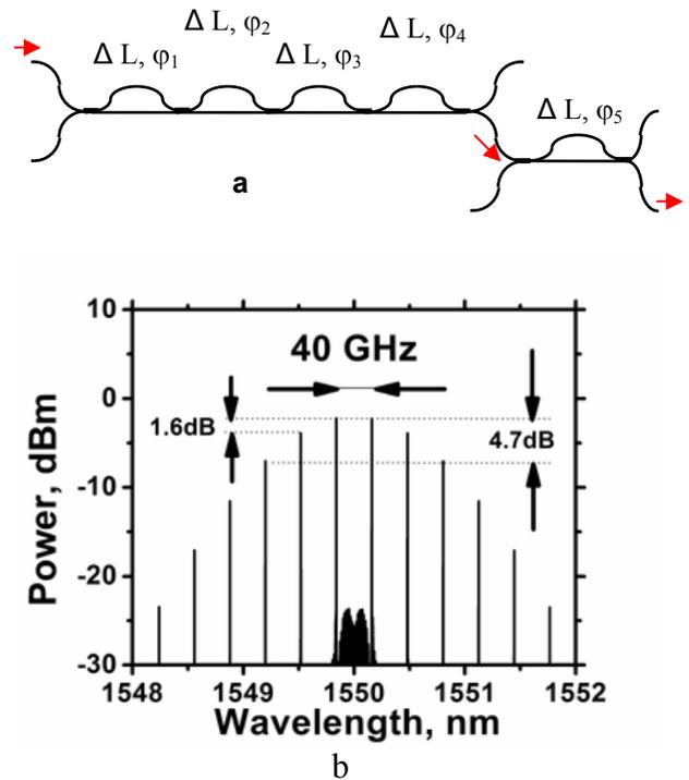
Figure 7. (a) Five-stage LF-MZI-2 for generation of optical signal at 40 GHz and (b) the optical output of the LF-MZI-2.
