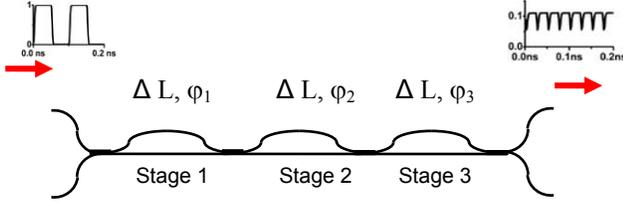
Figure 2. Three-stage LF-MZI for generation of optical signal at 40 GHz.
