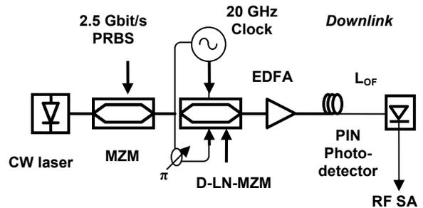
Figure 4. Simplified schematics of a ROF link with OCS using dual-arm  $\text{LiNbO}_3$ -MZM.
