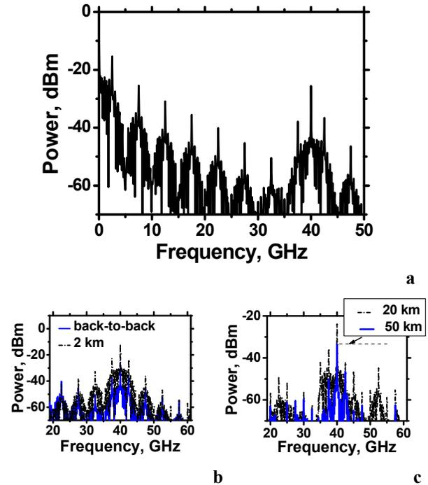
Figure 6. RF response of the photodiode in the proposed link: (a) back-to-back; (b) back-to-back and 2 km; and (c) 20 km and 50 km of the fiber link.
