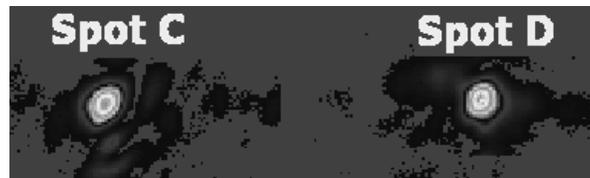
Fig. 3. Two output spots from the incoming B in the half-horn shaped deflector
