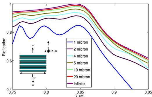
Fig. 4. Reflection of the SWG with different length of fingers
