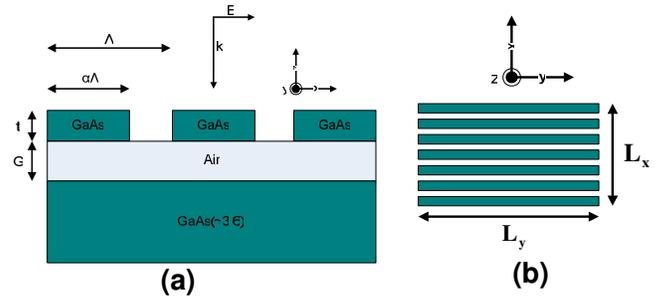
Fig. 1. SWG Structure a) Cross sectional view b) top view.
