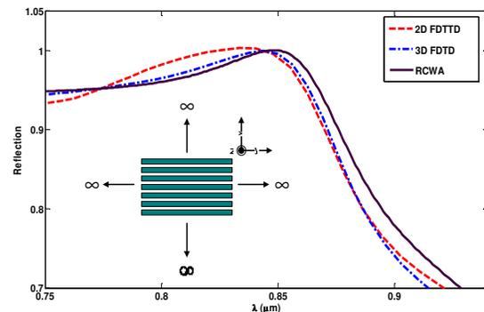
Fig. 2. Reflection of SWG using FDTD and RCWA.
