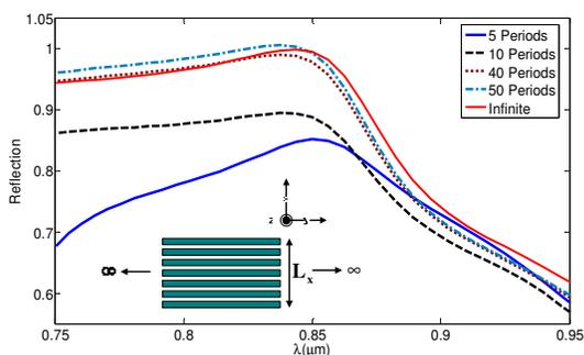
Fig. 3. Reflection of the SWG with different number of fingers
