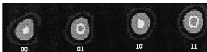
Fig. 2. Four output spots of the 1x4 optic switch.
