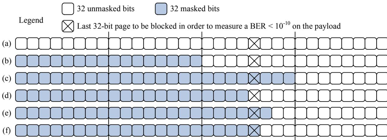
Fig. 2 Preamble length measurement using the non linear algorithm. The preamble length in this example is  $21 \times 32 = 672$  bits.
