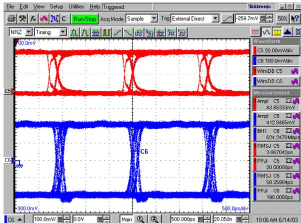
Fig. 3 Example of packet generation with a 160 ps phase step. A  $2^{11}$  PRBS at 622.08 Mbps was used.
