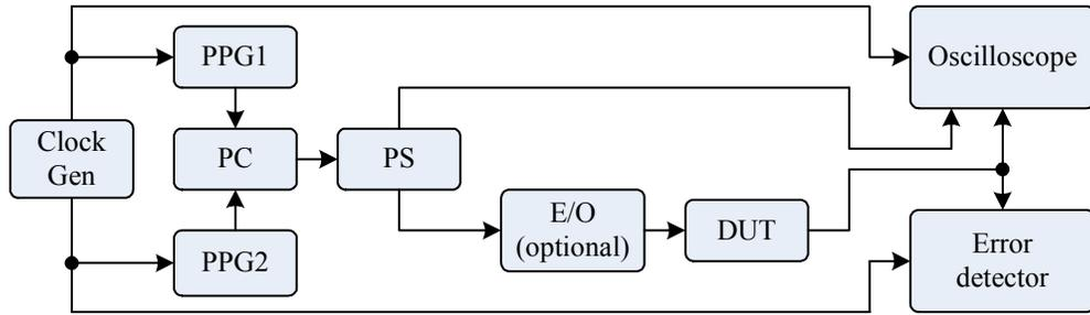
Fig. 1 Burst-mode test setup (the Matlab controller is not shown). PPG: pulse pattern generator, PC: power combiner, PS: power splitter.
