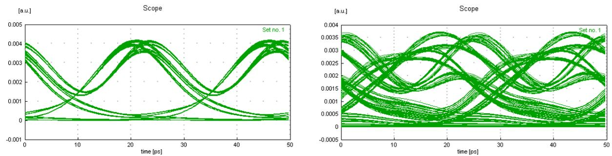
**Figure 6.** received 40Gb/s signals of a channel at the edge of the sub-band after passing one (left) and two (right) OADMs, channel spacing 100GHz.
