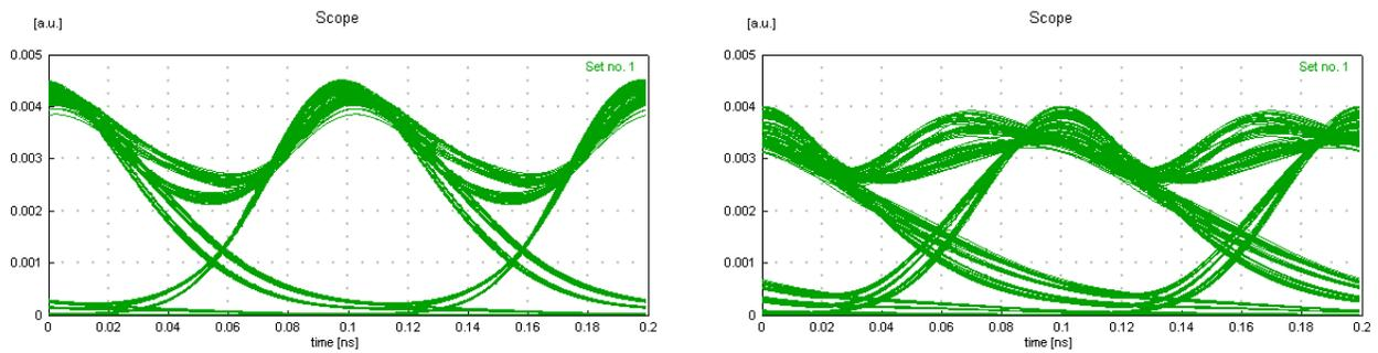
**Figure 11.** received 10Gb/s signals after passing four (left) and six (right) OADMs, channel spacing 100GHz, no band filter, no dispersion compensation.
