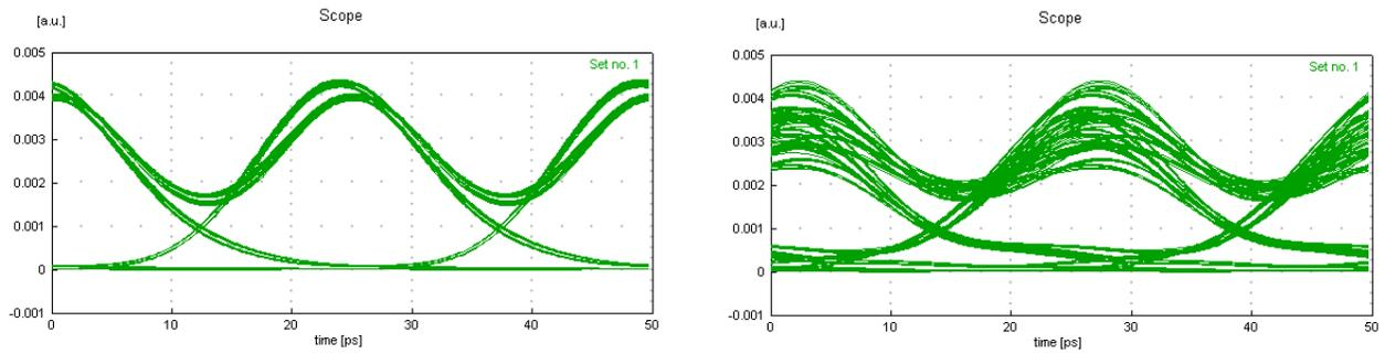
**Figure 5.** received 40Gb/s signals of a channel at the center of the sub-band after passing one (left) and three (right) OADMs, channel spacing 100GHz.
