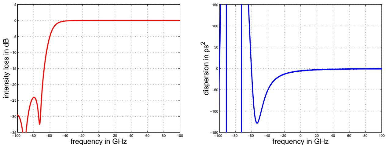
**Figure 2.** intensity loss and dispersion of a 100GHz optical filter in reflection.
