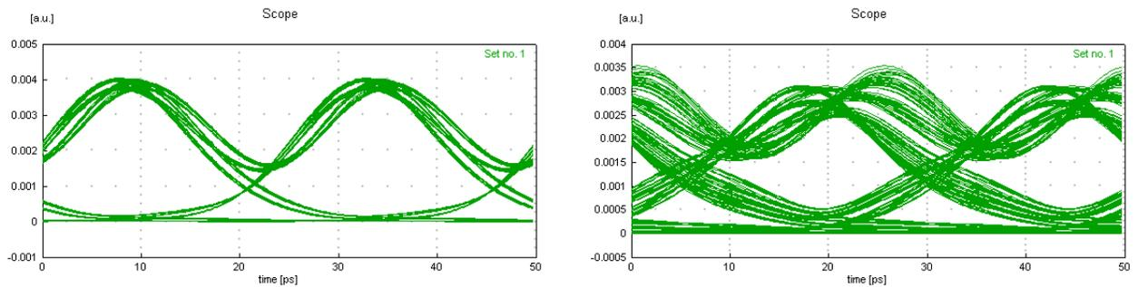
Figure 9. received 40Gb/s signals of a channel at the edge of the sub-band after passing one (left) and two (right) OADMs with dispersion compensation, channel spacing 100GHz.
