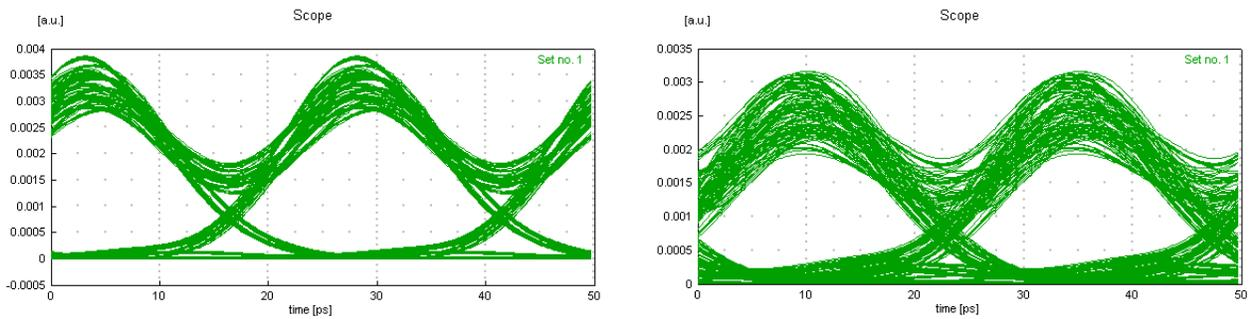
Figure 8. received 40Gb/s signals of a channel at the center of the sub-band after passing four (left) and eight (right) OADMs with dispersion compensation, channel spacing 100GHz.
