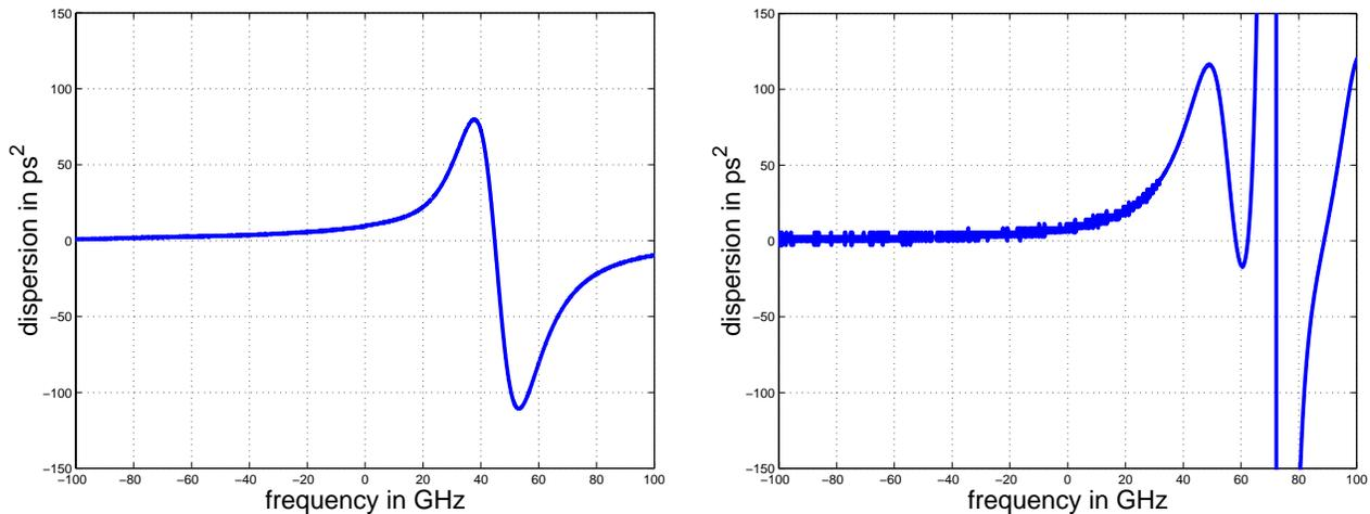
**Figure 3.** dispersion of 400GHz band filters. Left: the channel is at the “blue” edge of a band filter in transmission; Right: the channel is at the “red” edge of a band filter in reflection.
