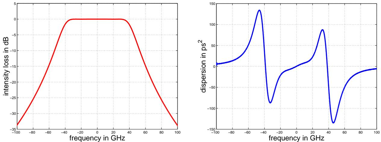
**Figure 1.** intensity loss and dispersion of a 100GHz optical filter in transmission.
