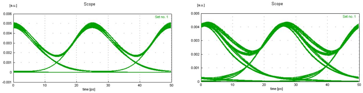
**Figure 10.** received 40Gb/s signals after passing four (left) and six (right) OADMs, channel spacing 200GHz, no band filter, no dispersion compensation.
