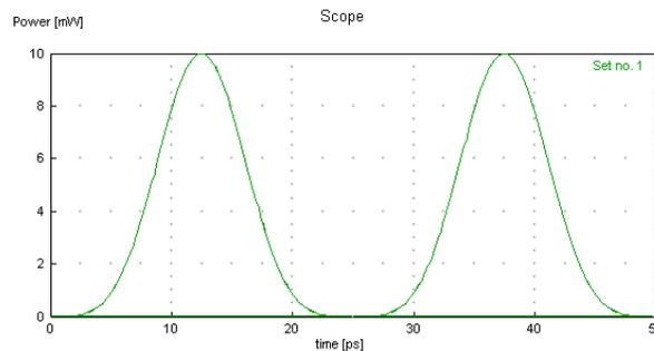
**Figure 4.** 40Gb/s chirp-free RZ optical pulses with 33% duty-cycle.
