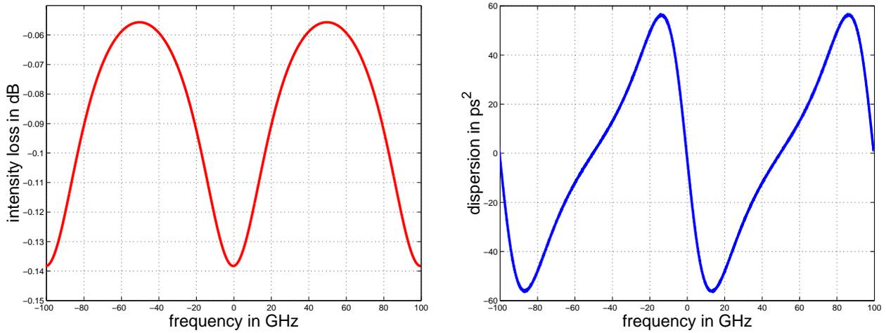
Figure 7. intensity loss and dispersion of an FP etalon.
