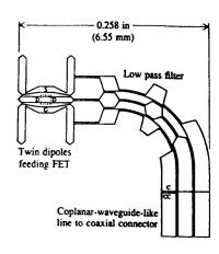
Millimeter Wave Radiation Comb Generated With Optical Pulse Train
