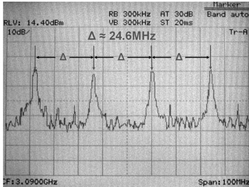
Fig. 6. Output spectrum of the PRBS generator. The separation of the peaks is the clock frequency divided by the PRBS sequence length.
