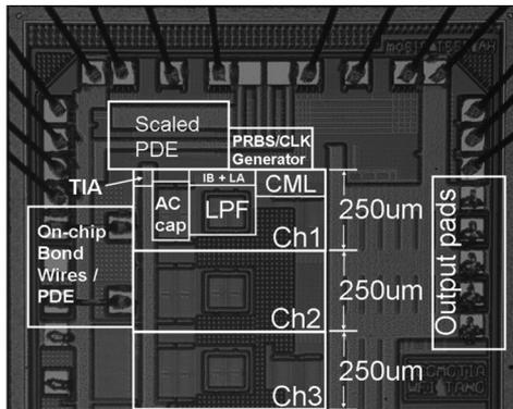
Fig. 3. Micrograph of a wirebonded die sample.
