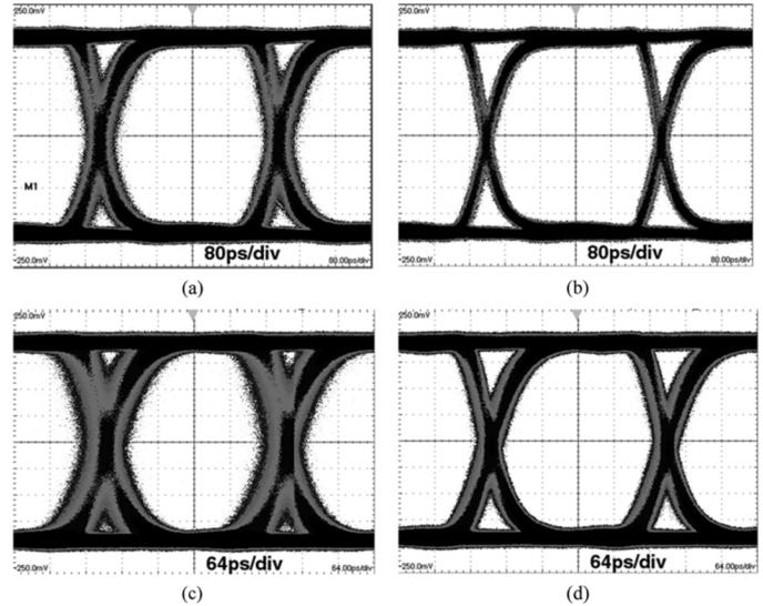
Fig. 4. Measured differential eye diagrams at 2.5 and 3.125 Gbit/s with single-channel operation. (Vertical:  $50 \text{ mV/div}$ ). (a) 2.5 Gbit/s,  $20 \mu\text{A}$  input. (b) 2.5 Gbit/s,  $220 \mu\text{A}$  input. (c) 3.125 Gbit/s,  $20 \mu\text{A}$  input. (d) 3.125 Gbit/s,  $220 \mu\text{A}$  input.
