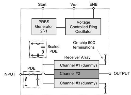
Fig. 1. Block diagram of the parallel optical receiver chip with on-chip clock and PRBS generators for crosstalk power penalty measurement.
