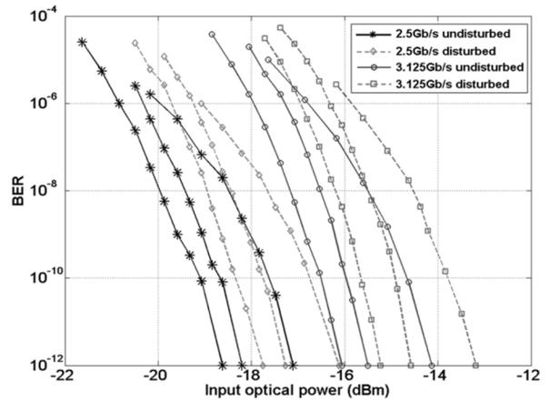
Fig. 7. Single-ended BER measurement results for 2.5 and 3.125 Gbit/s. Each group contains 3 BER curves which correspond to 3 different PRBS sequence lengths. From left to right: PRBS  $2^7-1$ , PRBS  $2^{15}-1$ , and PRBS  $2^{23}-1$ .
