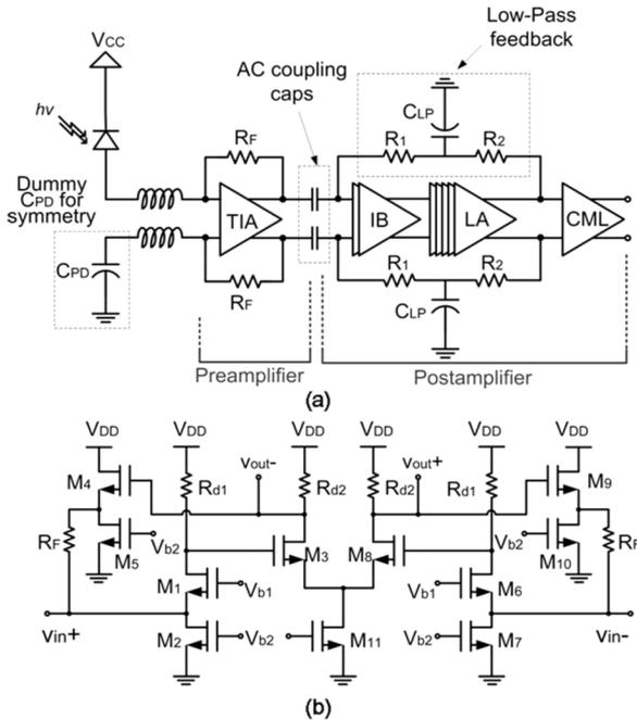
Fig. 2. (a) Block diagrams of one receiver channel; (b) TIA schematics.
