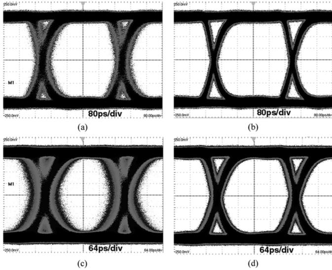
Fig. 5. Measured differential eye diagrams at 2.5 and 3.125 Gbit/s with adjacent channels turned on. (Vertical: 50 mV/div). (a) 2.5 Gbit/s, 20  $\mu$ A input. (b) 2.5 Gbit/s, 220  $\mu$ A input. (c) 3.125 Gbit/s, 20  $\mu$ A input. (d) 3.125 Gbit/s, 220  $\mu$ A input.
