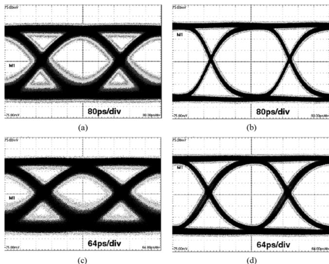
Fig. 8. Measured differential eye diagrams with 0.75-V supply for the post amplifier. (vertical: 15 mV/div). (a) 2.5 Gbit/s, 20  $\mu$ A input. (b) 2.5 Gbit/s, 220  $\mu$ A input. (c) 3.125 Gbit/s, 20  $\mu$ A input. (d) 3.125 Gbit/s, 220  $\mu$ A input.
