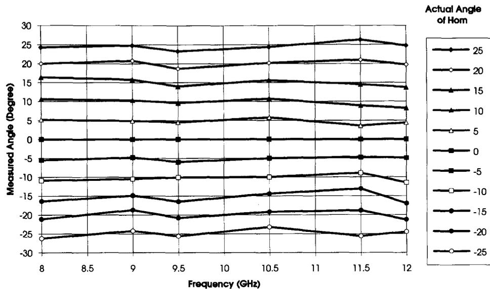
Fig. 3. Measured angle from  $-25$ – $25^\circ$  over an 8–12 GHz band exhibiting “squin free” operation measured in the symmetric configuration. Deviations of the measurements from the actual angle of the horn are attributed to random phase shifts in the cables, amplifiers, and mixers. Comparable data was achieved using the asymmetric system.
