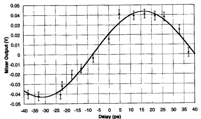
Fig. 2. Homodyne mixing output voltage versus optical delay time at 10.5 GHz with the X-band horn at  $-25^\circ$ . The least squares fit to the measured data determines the microwave phase delay,  $\Delta\varphi_m$ , with improved accuracy.
