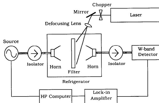
FIG. 3. Experimental arrangement used for optical response measurements.
